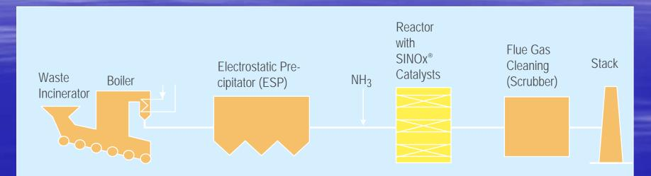
The flue gas from the boiler undergoes particulate dust removal with an ESP before
