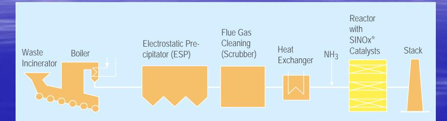
The catalyst is placed at the very end of the flue gas cleaning eqiupment, after the ESP and flue gas scrubber. The flue gas has to be reheated to the proper catalyst operating temperature.
